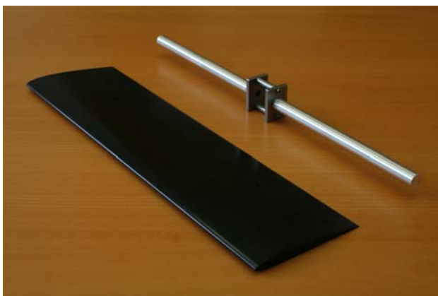
Fig. 4 SD7003 carbon-fibre profile and dummy cylinder shown for comparison; note cylinder identical to profile in mass ( \pm 0.5 g) and spanwise distribution
