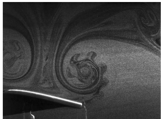
Fig. 6 Visualization depicting strong leading- and trailing-edge separation at bottom of stroke during a dynamic-tare measurement
